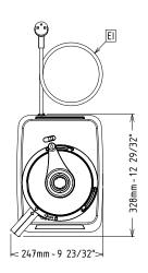
Electric Supply voltage: 220-240 V/1N ph/50/60 Hz Electrical power, max: 0.75 kW 0.75 kW **Total Watts:** Capacity: Performance (up to): Capacity: 2.6 litres Key Information: External dimensions, Width: 247 mm External dimensions, Depth: 328 mm External dimensions, 456 mm Height: **Shipping weight:** 18.7 kg Meat mincing capacity: 0 kg Mayonnaise preparation 0 kg capacity: **Pastry preparation**
